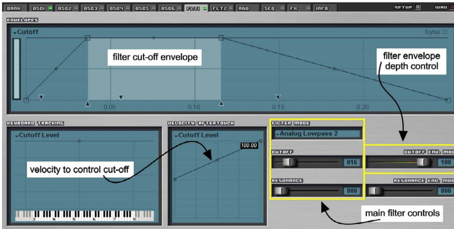
figure 32: setting up Rhino so that the filter cut off can be modulated by the filter envelope and velocity
